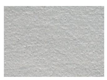
Efflorescence Coat over the substrate. Allow the Efflorescence Coat to dry for 2 – 3 hours. Over this normal coating / skim coat can be applied.
